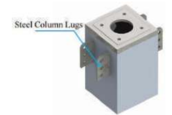
Steel Column Lifting Eye (with Connection Ear Plate)
