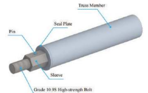
Truss Member Detail Drawing (2)
