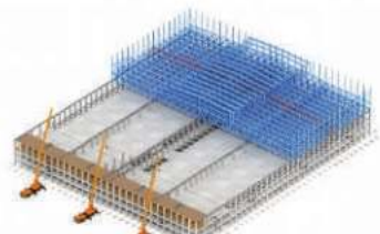
Positioning and Unloading of the Second Integrated Sliding Unit
