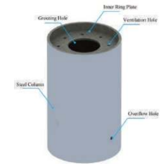
Steel Pipe Column Grouting Hole and Overflow Hole
