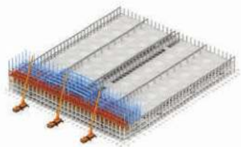
Sequential Completion of the First Integrated Sliding Unit
