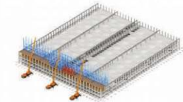
Installing Adjacent Two Truss Frames and Connecting Them to the First Unit
