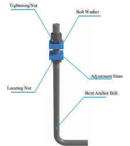
Foundation Bolt Installation Schematic
