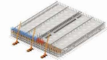
Sequential Installation of Trusses to Form Stable Units
