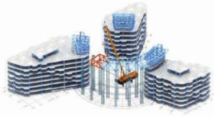
Continuous Installation of Formwork Support Scaffolding and Truss Units
