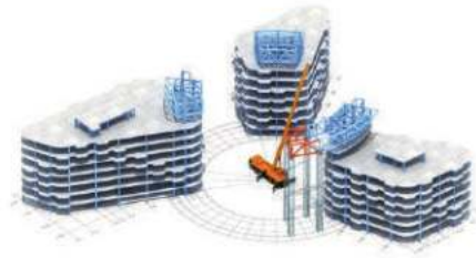
Formwork Connection and Installation of Truss Units
