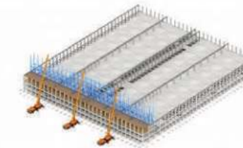
Sliding the First Installation Unit Truss (Two Frames)
