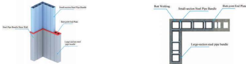
Steel Pipe Bundle Variable Section Connection Node Isometric Drawing
