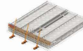
On-Site High-Altitude Assembly of the First Section of Trusses
