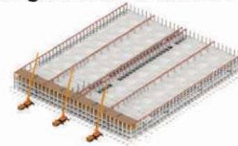
Erection of High-Altitude Assembly Platforms on Floors or Ground
