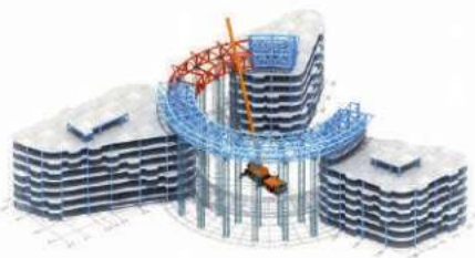
Sequential Installation of the Second Section of Aerial Trusses
