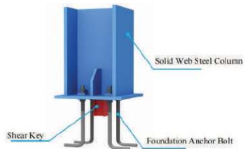
Steel Column Axonometric Detail Drawing
